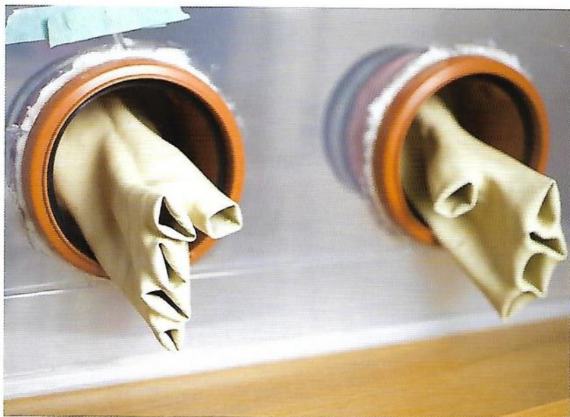
Turn the gloves of the glove box outwards like this when not in use.
