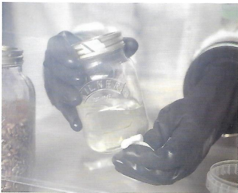
When using a glove box, wipe everything with a 10% bleach solution before use.
