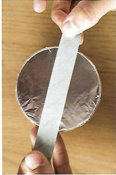
Autoclave tape holds foil on top of the jars and creates injection sites.
