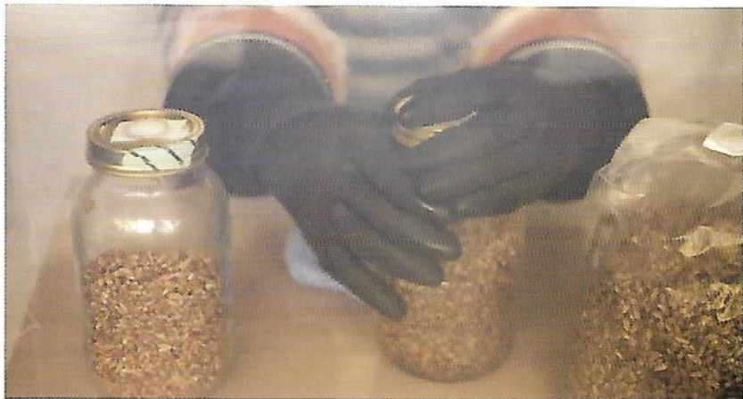
Grain-to-grain transfers should take place in a flow hood or glove box, like this.
