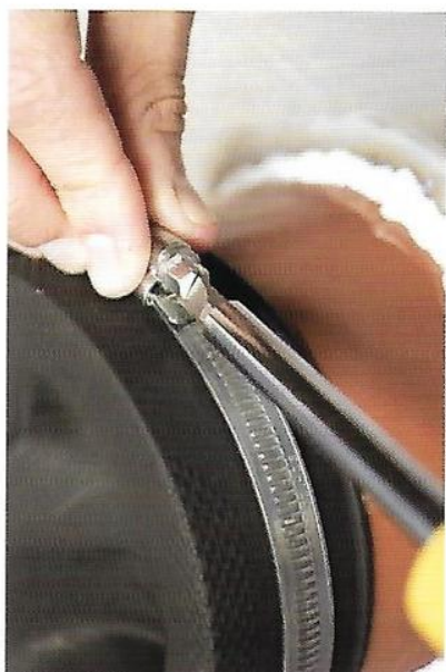
24. Turn the screw to tighten the Jubilee Clip and secure the glove.
