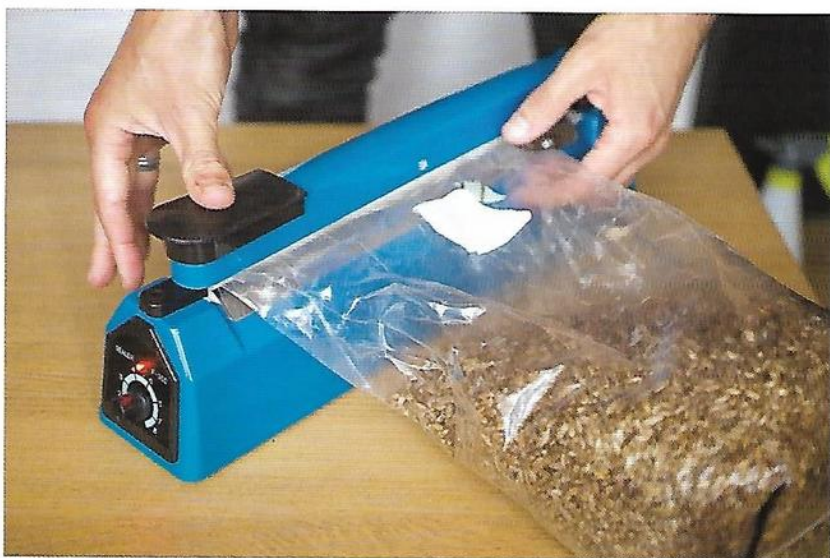
After transferring to grain bags, an impulse sealer will help keep an airtight seal.
