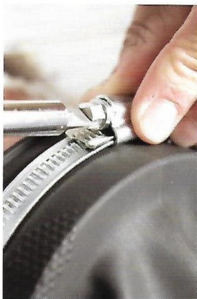
25. Repeat this with the second Jubilee Clip. Ensure the gloves won't come off.
