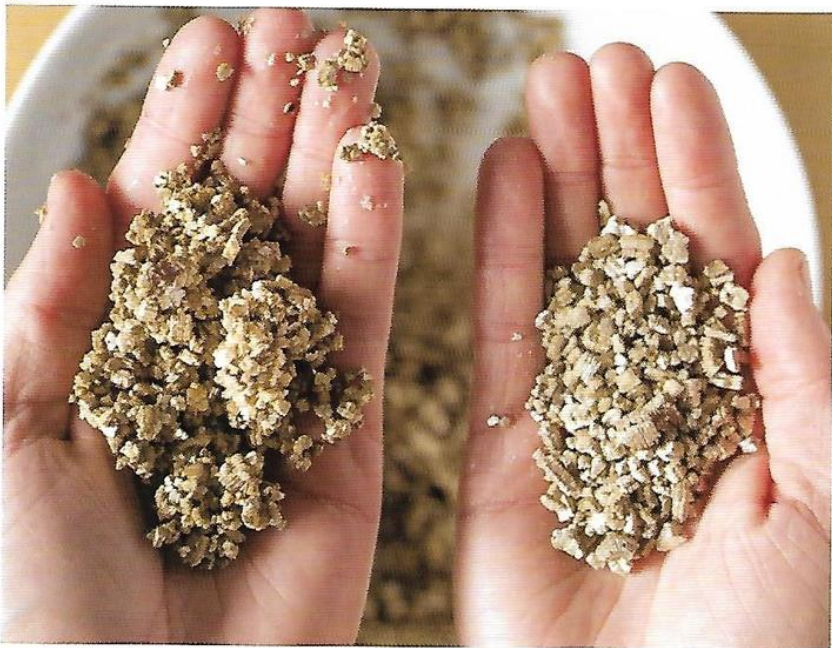
10. This is what properly hydrated vermiculite looks like (left hand).
